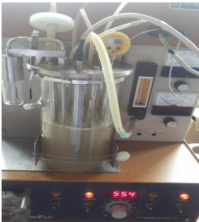
Figure 7. New Brunswick Scientific BioFlow C-32 fermenter (1.5 L) showing the reaction containing resting cells of APB-6 for the biotransformation of butyramide to butyhydroxamic acid
