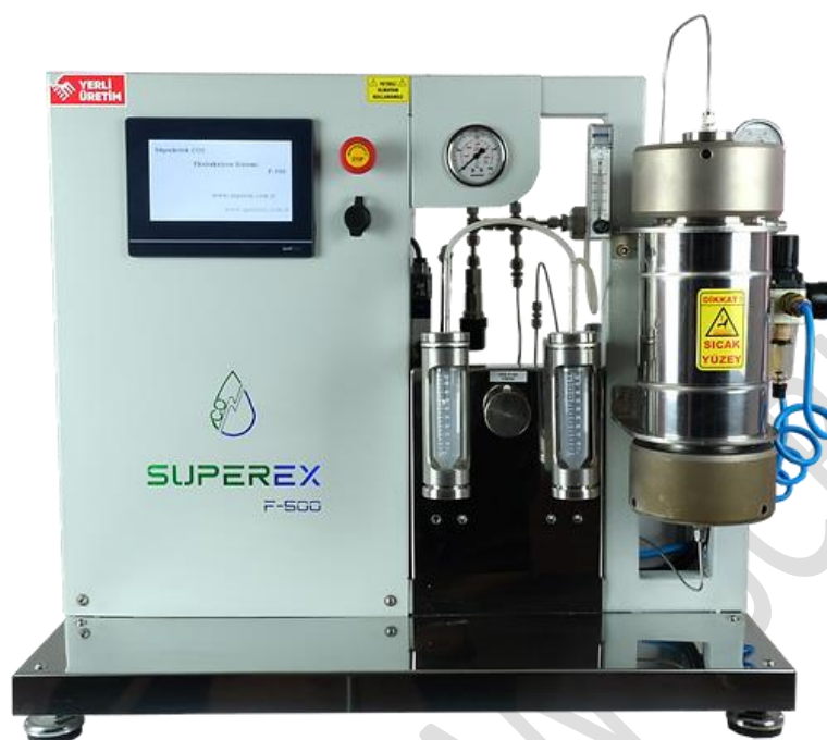
Figure 1. Supercritical CO 2 extraction device used to obtain the terebinth fruit extracts.
